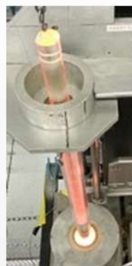
Fig 2: Polymer fiber drawing tower in the lab
