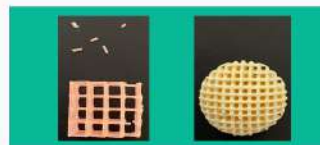
Fig. 5. Appearance of cube and sphere structure after vigorous stirring.
