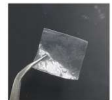
Fig. 1. Samples of PMMA SPE film trimmed out from the dried electrolytes film.
