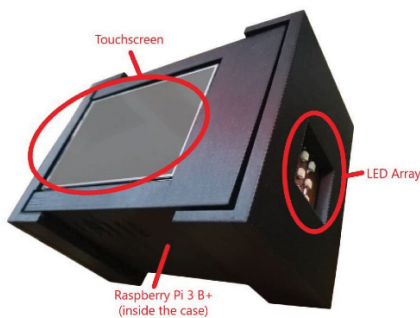
Fig 5. VLC transmitter prototype with integrated touchscreen.
